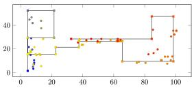
Fig. 3. Live Test: K\* algorithm predicting position as the researcher walks the path in black allowing the device to change orientation. Color indicates time starting at blue, ending at red with smooth interpolation between.
